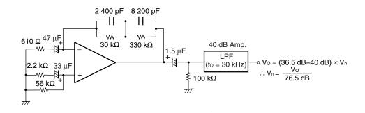
Figure3 Noise Measurement Circuit (FLAT+JIS A)
