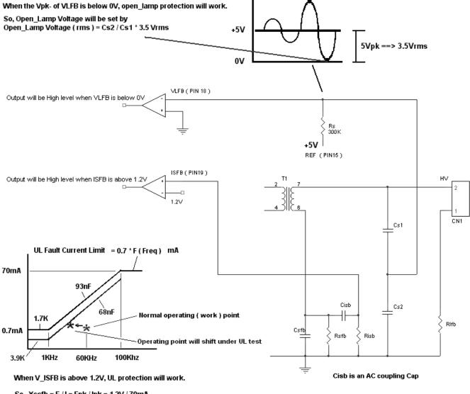
So, Xcsfb = E / I = Epk / Ipk = 1.2V / 70mA Xcsfb = 1 / ( 2 \* 3.14 \* F\* Csfb ), F = 100K Csfb = 1/ ( 2 \* 3.14 \* 100K \* Xcsfb ) = 70mA / ( 2 \* 3.14 \* 100K \* 1.2V ) = 93nF Get Csfb\_max = 93nF , therefore Csfb is selected below 93nF approx 75nF or 68nF.
