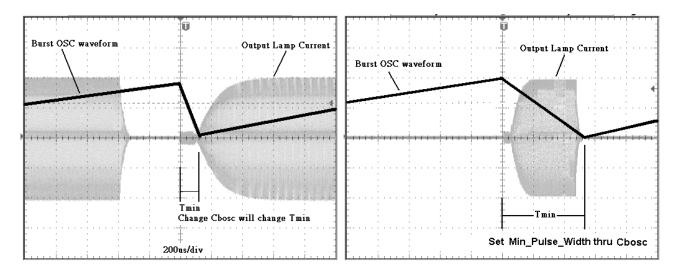
Figure 4: Burst Oscillator Waveform versus Output Lamp Current
