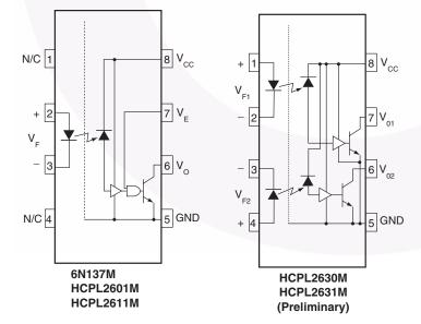
A 0.1 $\mu$ F bypass capacitor must be connected between pins 8 and 5<sup>(1)</sup>.
