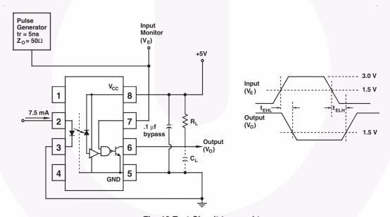
Fig. 13 Test Circuit  $t_{\text{EHL}}$  and  $t_{\text{ELH}}$
