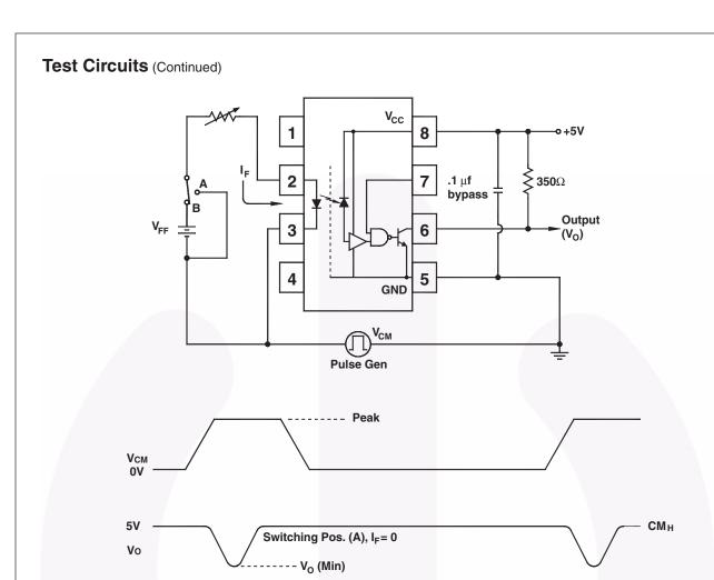
Fig. 14 Test Circuit Common Mode Transient Immunity
