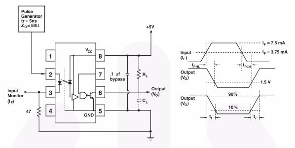
Fig. 12 Test Circuit and Waveforms for  $t_{\text{PLH}},\,t_{\text{PHL}},\,t_{\text{r}}$  and  $t_{\text{f}}$
