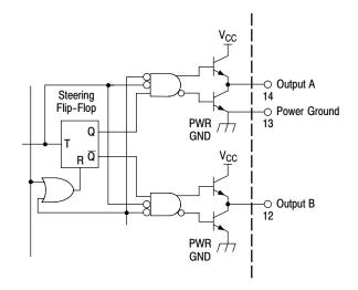
Figure 18. Steering Flip-Flop and Output Drivers
