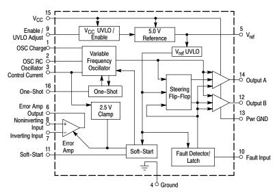
Figure 1. Simplified Block Diagram
