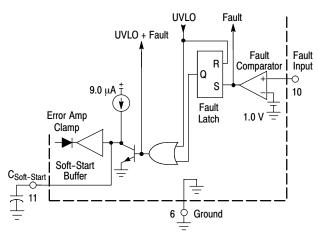
Figure 20. Fault Detector and Soft-Start
