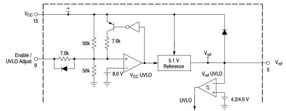
Figure 19. Undervoltage Lockout and Reference
