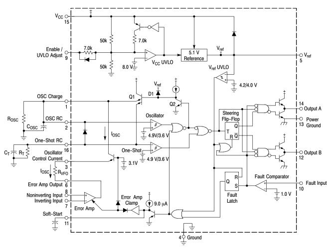
Figure 14. MC34067 Representative Block Diagram
