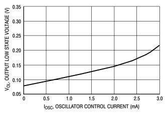
Figure 4. Error Amp Output Low State Voltage versus Oscillator Control Current
