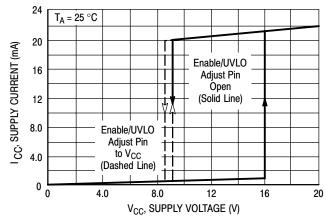
Figure 13. Supply Current versus Supply Voltage
