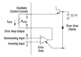
Figure 17. Error Amplifier and Clamp
