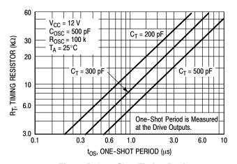
Figure 5. One-Shot Timing Resistor versus Period
