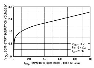
Figure 11. Soft-Start Saturation Voltage versus Capacitor Discharge Current
