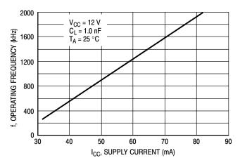
Figure 12. Operating Frequency versus Supply Current
