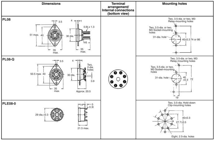
Note: When mounting, pay due attention to the direction of the key groove of applicable Relays.
