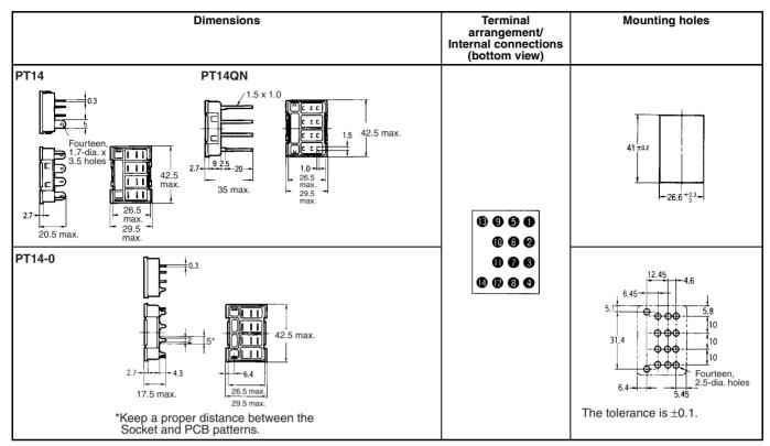
Note: Use a panel with a thickness of 1 to 2 mm when mounting a Socket on it.
